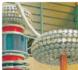
*High Voltage Test Transformer
