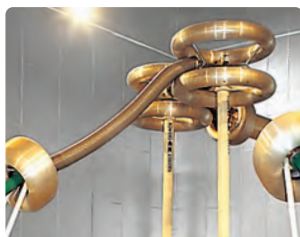
*Partial discharge Test Equipment
